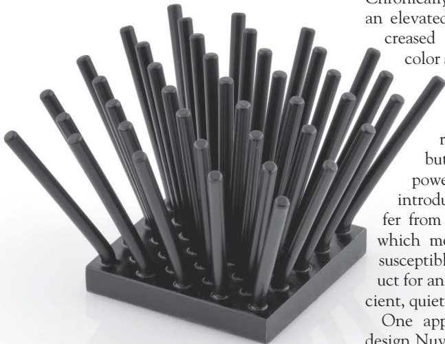
Figure 3 Cool Innovations' flared-pin fin heat sinks feature an array of sparsely configured round pins that slant outward, a configuration that can cool the HB-LED die in SSL in natural-convection environments.
