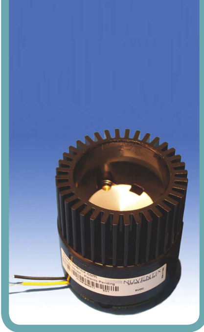
Figure 2 Nuventix cooling devices consist of a diaphragm mounted in a cavity. An electromagnetic driver vibrates the diaphragm 100 to 200 times per second, forcing tiny jets of air out through openings in the cavity. These devices are virtually silent compared with conventional fans.
