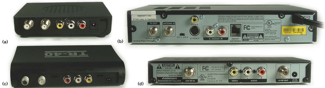
Figure 3 Back-panel perspectives of Access HD's DTA-1080D (a), Apex Digital's DT502 (b), Dish Network's TR-40 CRA (c), and Sansonic's FT-300A (d) reveal the hardware enhancements that Apex Digital's product provides.
